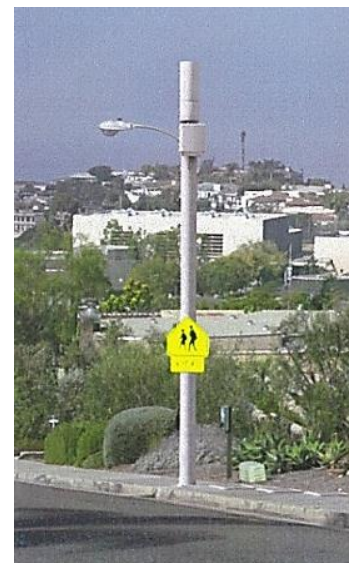
Visualization of Laguna Beach's approved small cell street light design
